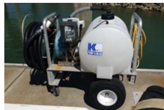
In-slip pumpout tank at Oyster Cove Marina Photo by SFEP
